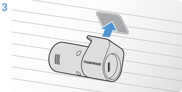
Attach the product with the THINKWARE logo facing indoors and press the adhesive tape firmly to secure the camera.
