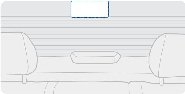
Select a location on the rear windshield where there is no defrost grid wire and the camera can record the entire rear view.
