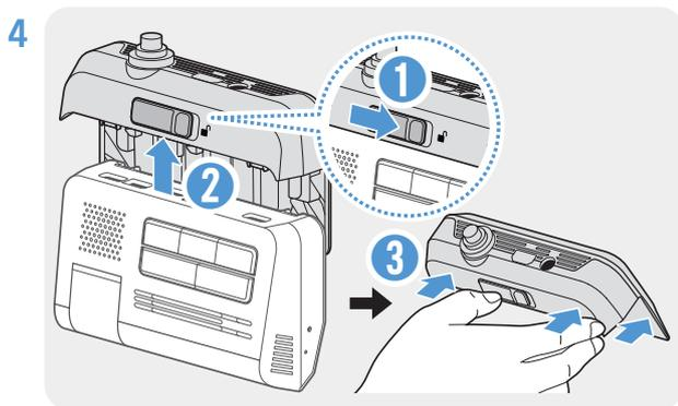
Pull the slide lock to the right and pull up the cradle to remove it from the product. Then push the cradle against the windshield to ensure that it is firmly fixed.
