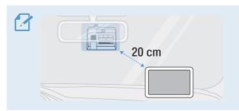
If a GPS navigating device is installed on the dashboard, its GPS reception may be affected depending on the dashboard camera's installation location.
