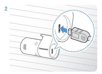
Connect the other end of the rear camera cable to the rear camera's connection port.
