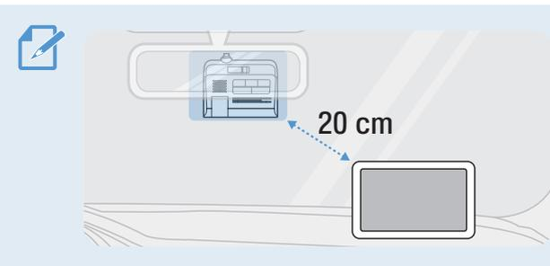
If a GPS navigating device is installed on the dashboard, its GPS reception may be affected depending on the dashboard camera's installation location. Adjust the installation location of the GPS navigating device to ensure that the two devices are separated by at least 20 centimeters (approximately 8 inches).
