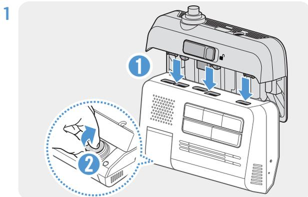
Align the cradle with the mount rail and connector on the product and slide it down until you hear a click. Then, carefully remove the protective film.
