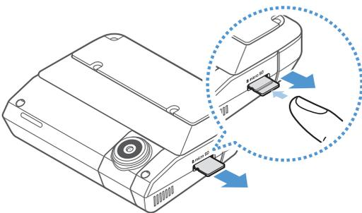
Before removing the memory card, ensure that the product is turned off. Gently push the bottom of the memory card with your fingernail to release it, and then remove it from the product.
