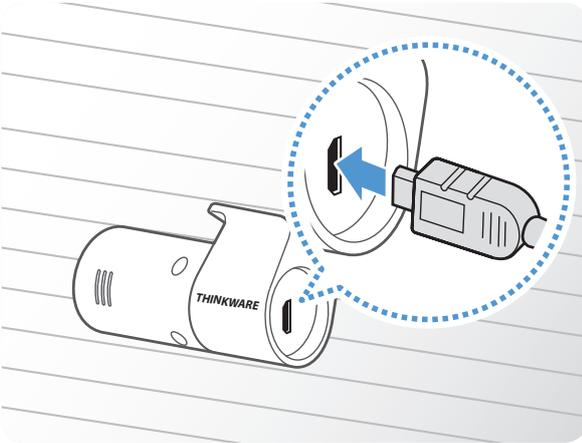
Connect the other end of the rear camera cable to the rear camera's connection port.
