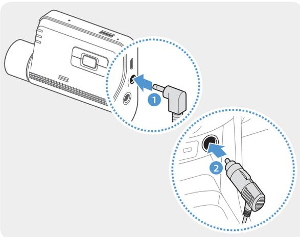
Connect the car charger to the product's DC-IN power port and insert the cigar jack into the vehicle's power socket.
