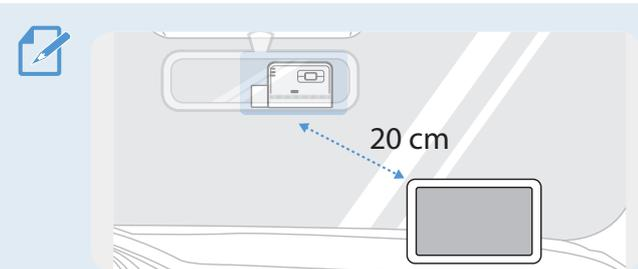
If a GPS navigating device is installed on the dashboard, its GPS reception may be affected depending on the dashboard camera's installation location. Adjust the installation location of the GPS navigating device to ensure that the two devices are separated by at least 20 centimeters (approximately 8 inches).
