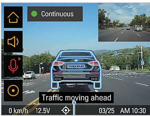
An alarm is output 4 seconds after the vehicle ahead has departed.
